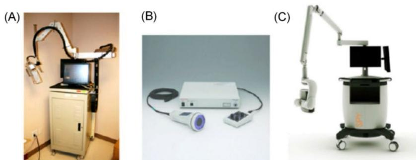
**Figure 1.** Commonly used near-infrared fluorescence imaging devices. (A) Frequency-domain photon migration (FDPM) imager, (B) Photodynamic eye, (C) SPY device. Adapted from Zhu B et al. *Br. J. Radiol.* 2015 Jan;88(1045):20140547 [54].
