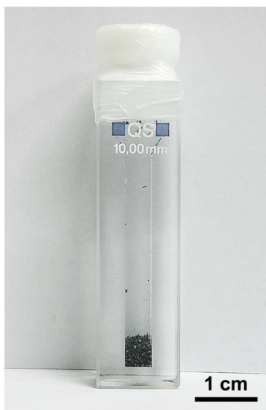
Figure S8. Photograph of a quartz cuvette containing the microcapsules at the bottom.
